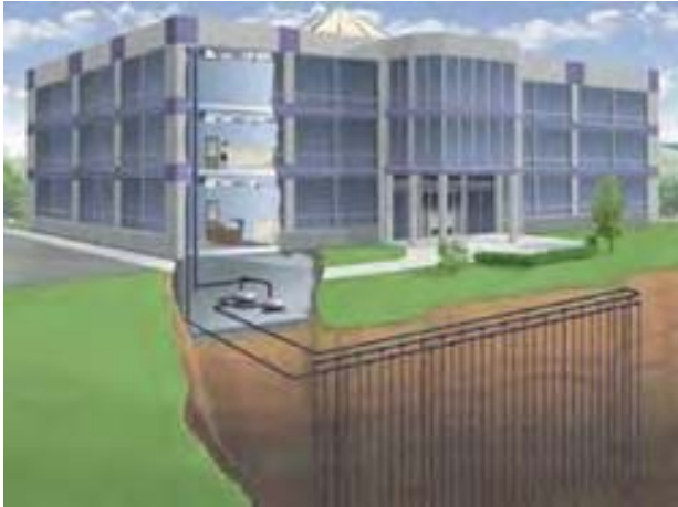
Closed Loop Wells Typically Higher First Cost (more wells) w/ Lower Maintenance Cost
